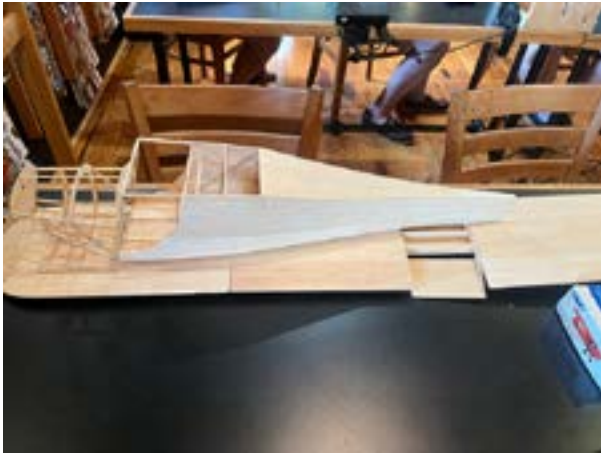
Jim Brode's Taylorcraft Airplane, An old kit by Comet. In lieu of tissue covering, Jim is using 1/32 balsa.
