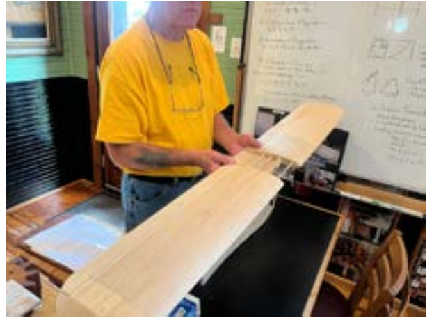
Jim Brode's Taylorcraft Airplane, An old kit by Comet. In lieu of tissue covering, Jim is using 1/32 balsa.
